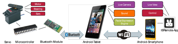
Figure 2: Control concept of remote-controlled rabbit.
