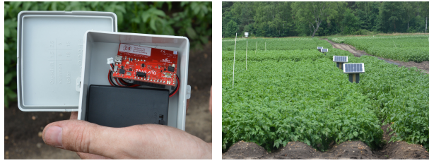
(a) INGA Node with Battery and (b) Deployed Base-Stations in the Potato Field
