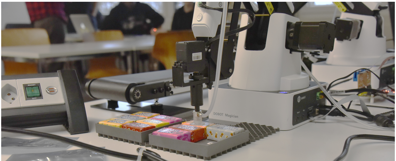
Figure 1: Snack-o-Mation in action during a TecDay event: students automate two Dobot Magician robots and a conveyor belt to deliver small sweets. This is a cooperative task where multiple teams are responsible for a single task in the automation system. Picture courtesy of Kantonsschule Zürcher Unterland, Bülach, Switzerland.
